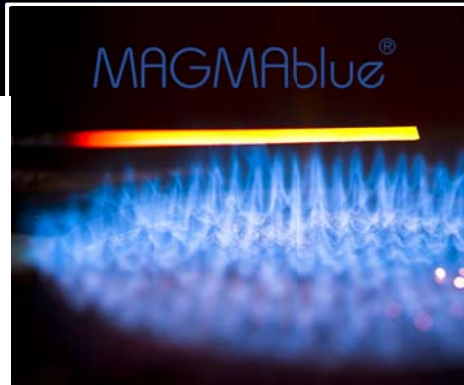
Example of a LOW-NO x gas flame as premix burner
